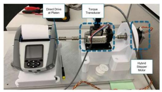
There is a Texas Instruments motor driver which is controlled by software on the attached PC. There is also a Transducer data acquisition unit for the transducer which runs on the same PC with different software.
