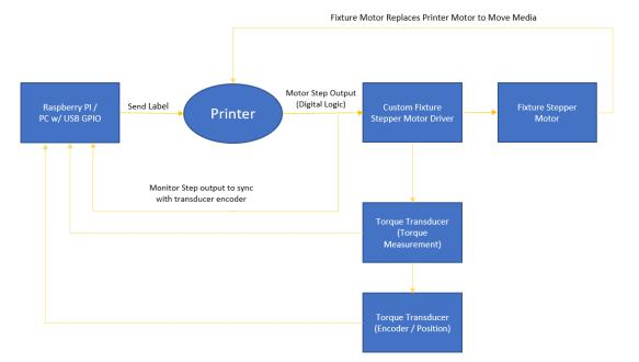
There will also be a second configuration of the fixture setup, that will be used to test stepper motor torque output. This setup will mount a small bipolar stepper motor that is used inside of our printers, and a magnetic particle brake on each side of the transducer. The stepper motor will be driven, and a load will be applied with the particle brake.
