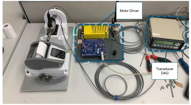
Currently we setup the motor driver software to run at our target speeds, and we begin feeding blank paper, and start the Torque transducer. With the current setup we get good information, but we do not capture the effects of the printhead sticking to the paper.
