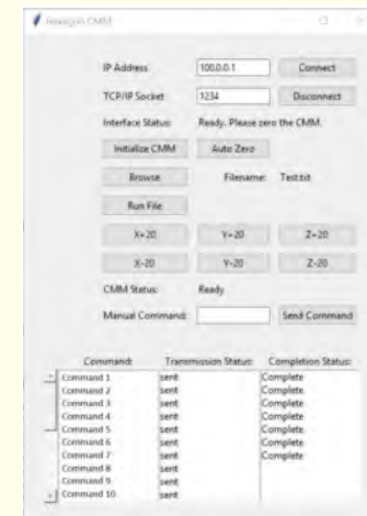
Fig. 4: This is a sample of the client interface in its current state during development. The interface provides the methods for the user to interact with the 3D printer retrofit.
