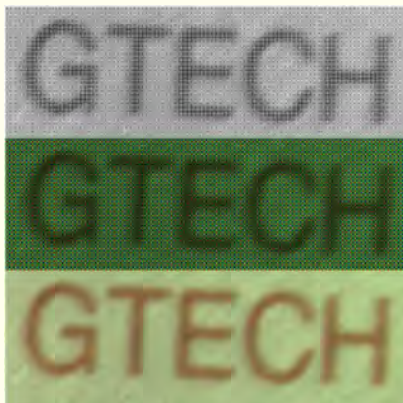
Fig. 2. Camera Output passed through our software: Raw sensor data (top) passed through a bayer filter (middle) with missing color values interpolated (bottom)
