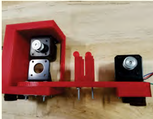
Fig. 2. Current iteration of prototype actuator. Stepper motors are connected to the base with pulleys in order to turn mirror screws without obstructing laser output.
