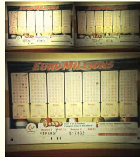
Fig. 4. Overexposed image (top left) and underexposed image (top right) combined to generate HDR image (bottom)
