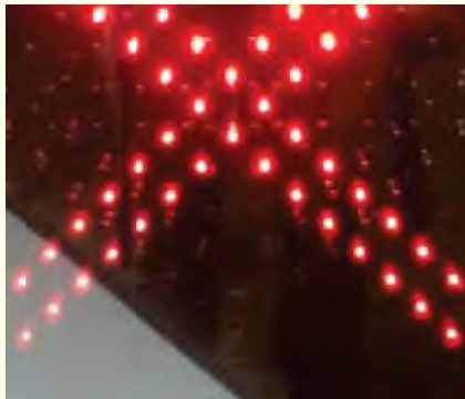
Fig. 1. Blank Out- Signs that are to be retrofitted with the cellular module to allow connection to the internet for change of message.
