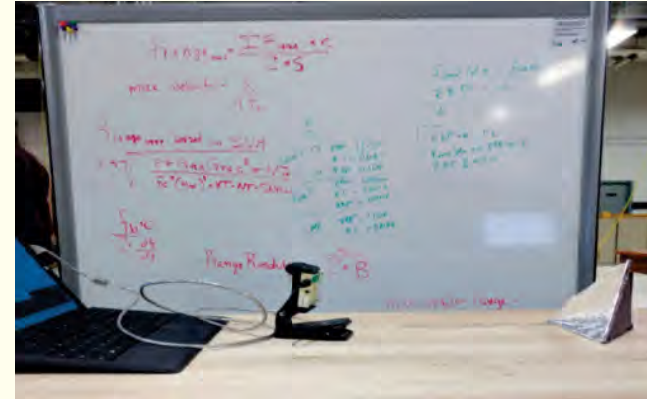
Fig 3. The radar board pointed at a corner reflector, with the radar range equations in the background.
