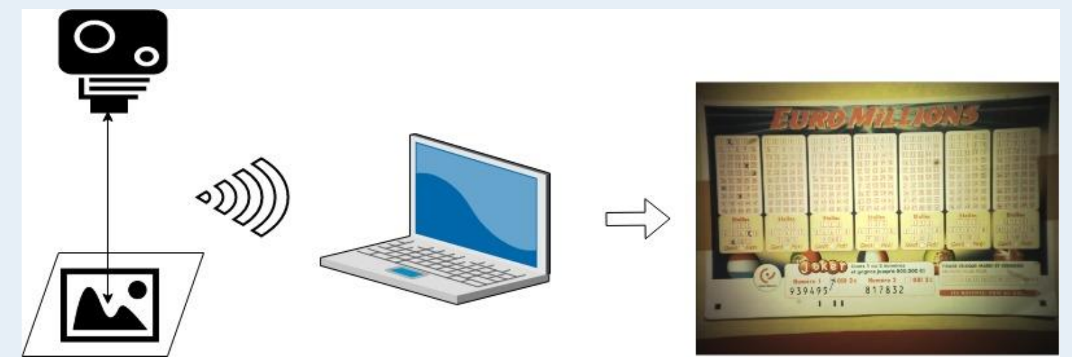
Figure 3: The process of producing HDR images: one or more over- and under- exposed photos are taken from the camera, and transferred wirelessly to the laptop for image processing applications; hence one high quality HDR image is produced.
