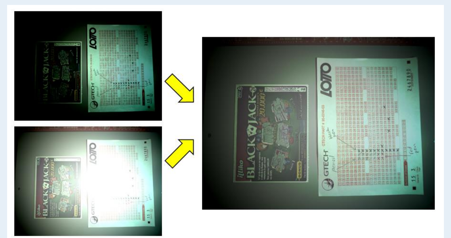
Figure 5: Underexposed (top left) and overexposed (bottom left) images combined using a contrast based HDR algorithm to produce an optimal quality HDR output image (right).
