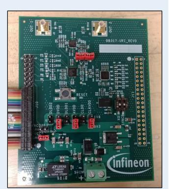
Figure 4: Waveform Generator Board
