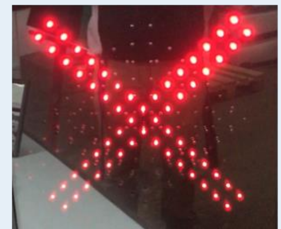
Fig. 2. Blank Out- Signs that are to be retrofitted with the cellular module to allow connection to the server for receiving a new message.
