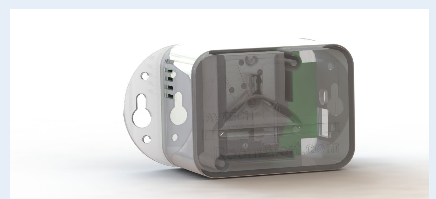
Fig. 4. Final enclosure with the sensor and blower
