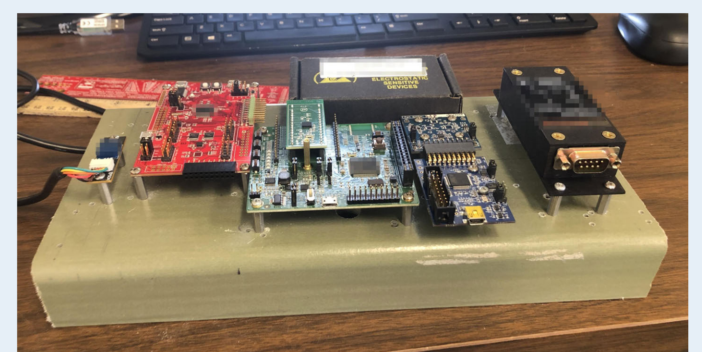
Fig 3: Boat Test Sensor Mount - Sensors Aligned for Maximum Accuracy
