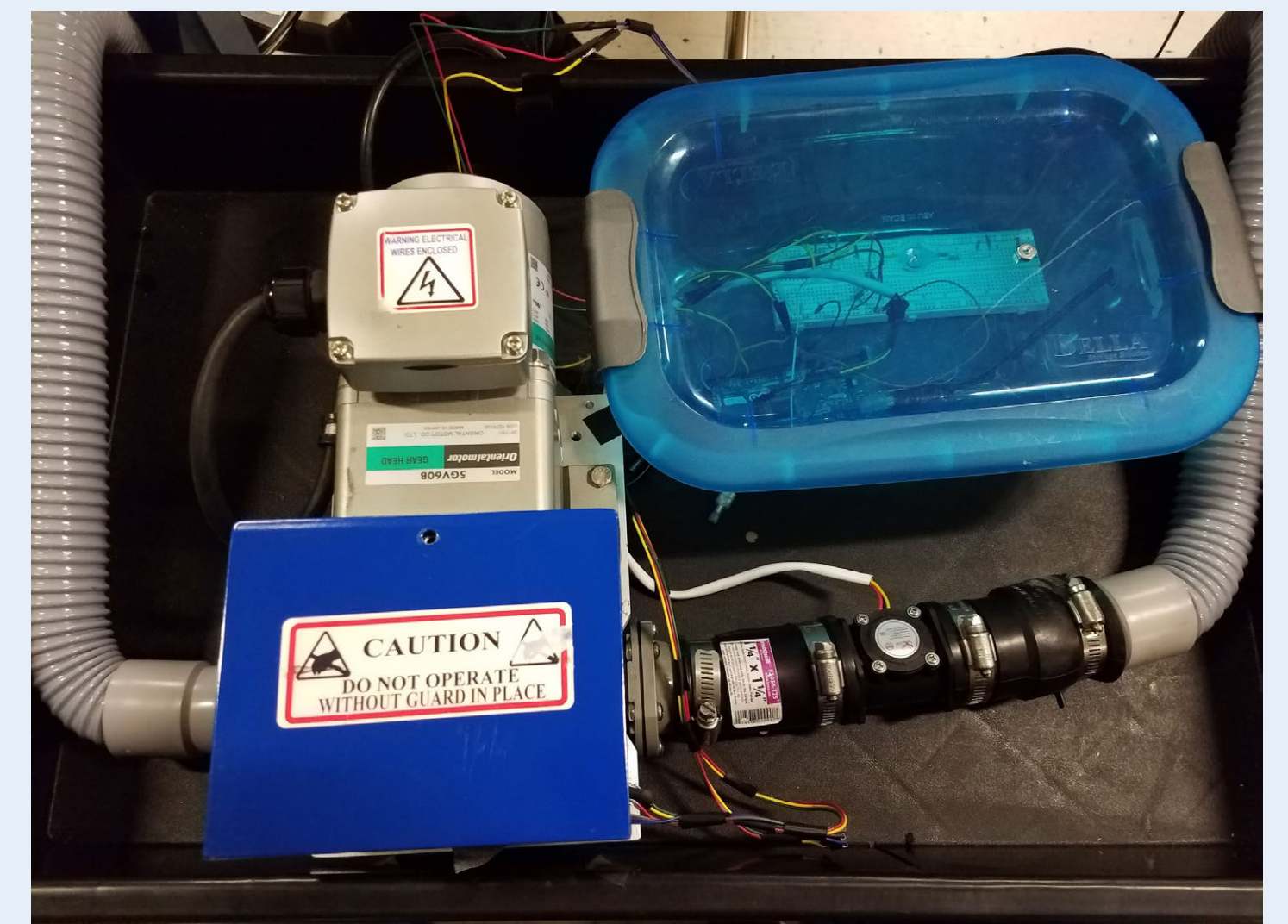
Fig. 3: View of pump, flow rate sensor, and microcontroller inside box.
