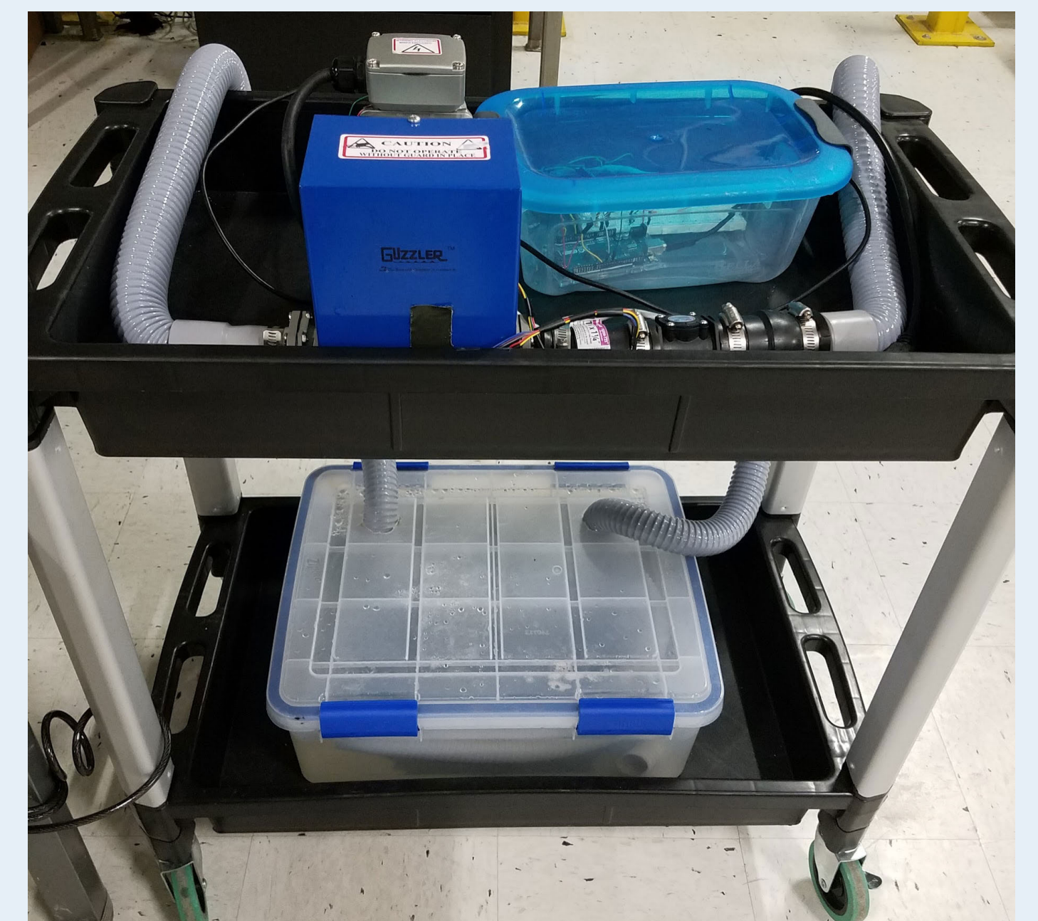
Fig. 4: Cart with water tank on bottom and pump with electronics on top.
