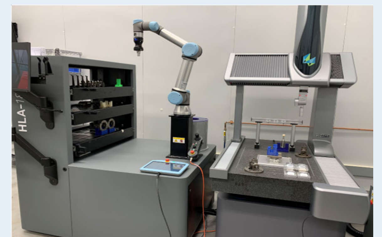
Figure 1. Robot Cell Setup with Coordinate Measuring Machine
