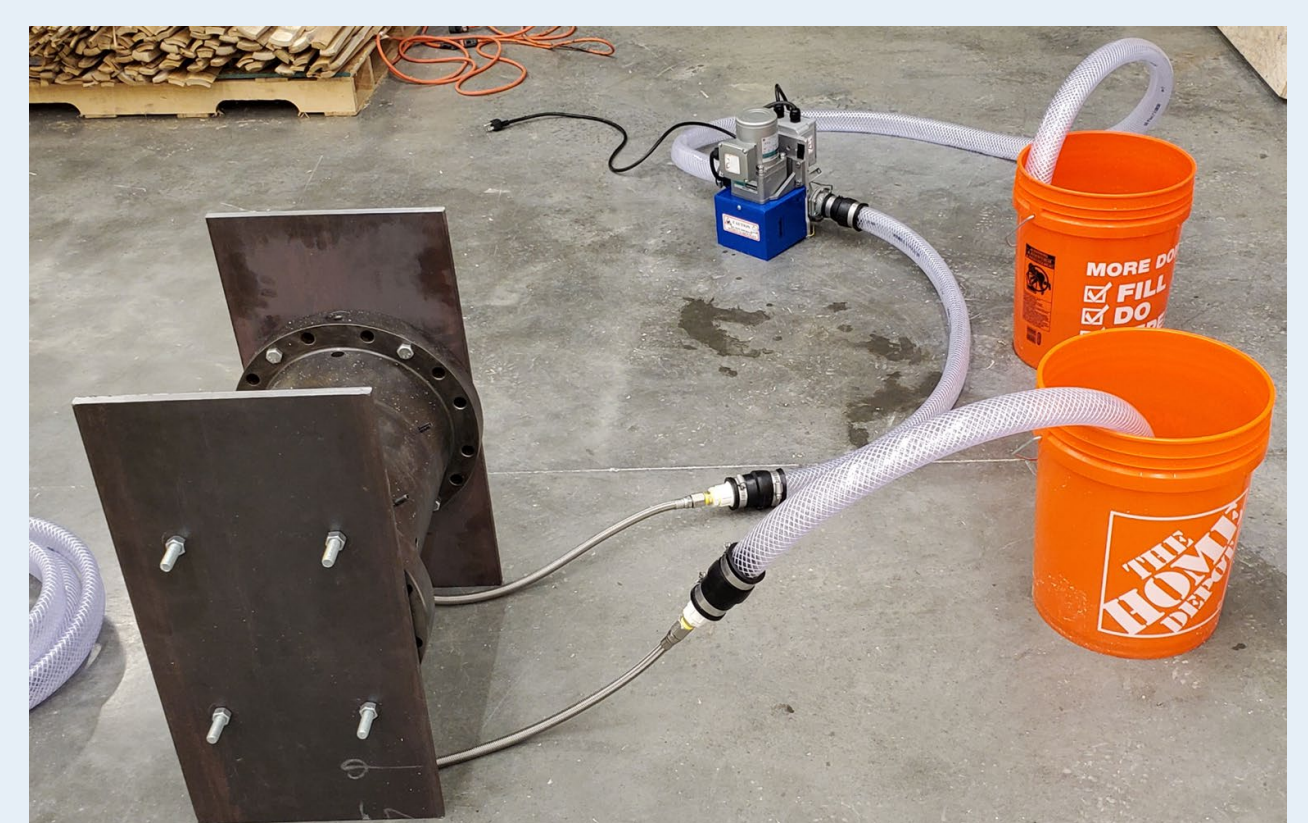
Fig. 4 - Zone with attached cooling system.
