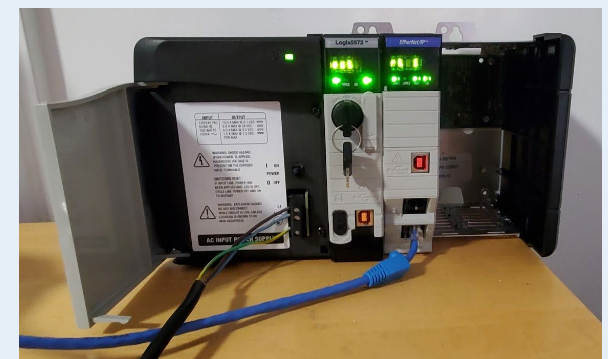
Fig. 2 - Programmable Logic Controller with, from left to right, the Processor and the Ethernet card.
