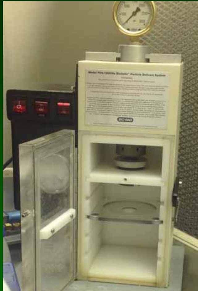
Biolistic PDS-1000/ He Particle Delivery System Catalogue number 165-2257 BioRad
