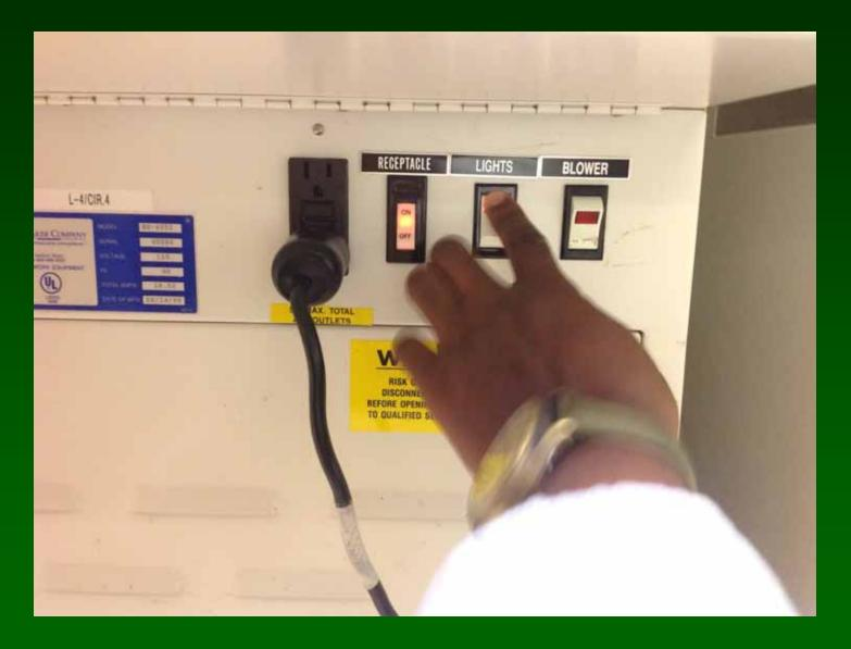
Receptacle (for microscope or other electrical), Lights and Blower switches are underneath to the right light. Blower is left on for routine use.
