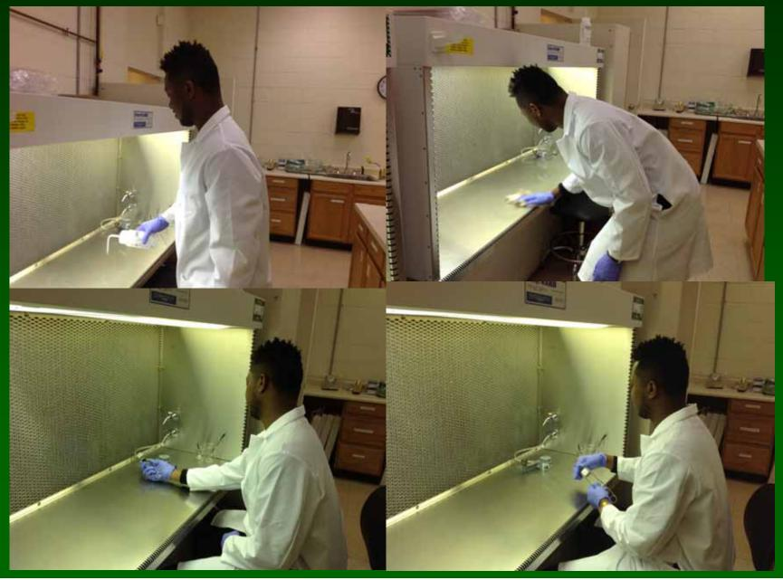
Also use 70% Ethanol on a paper towel to decontaminate any equipment in the hood, such as the dissecting microscope (knobs base and fiber optic cord or any other surface which may have been touched previously)
