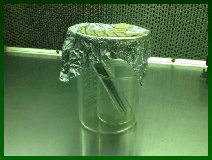
Forceps, scalpels, spatulas in a glass test tube, which can be used for the 95% alcohol used to flame or bead sterilize
