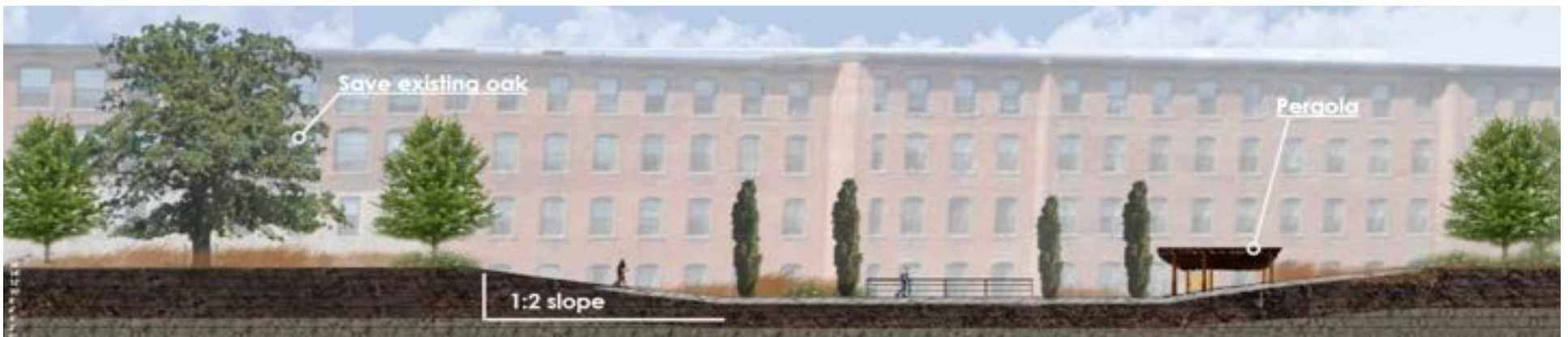
Cross section of park 8' elevation change
