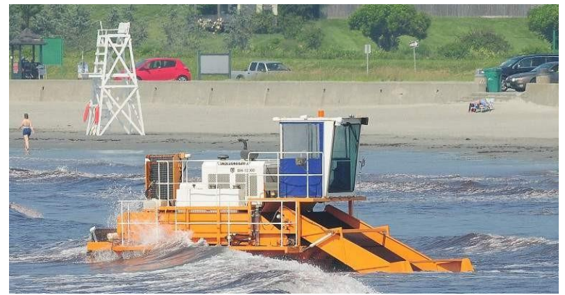
Seaweed harvester used on Easton Beach to improve water quality (photo credit: Newport Daily News)
