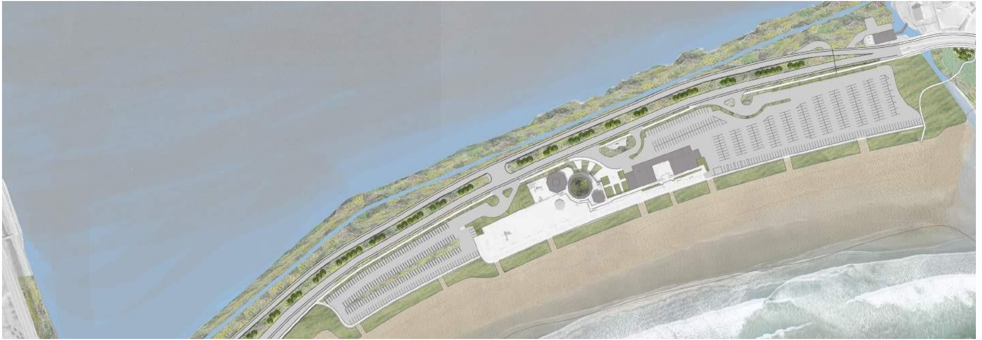
Victoria Bockstael: Design in plan view showing reorganized parking and green space as well as biofiltration areas for stormwater runoff
