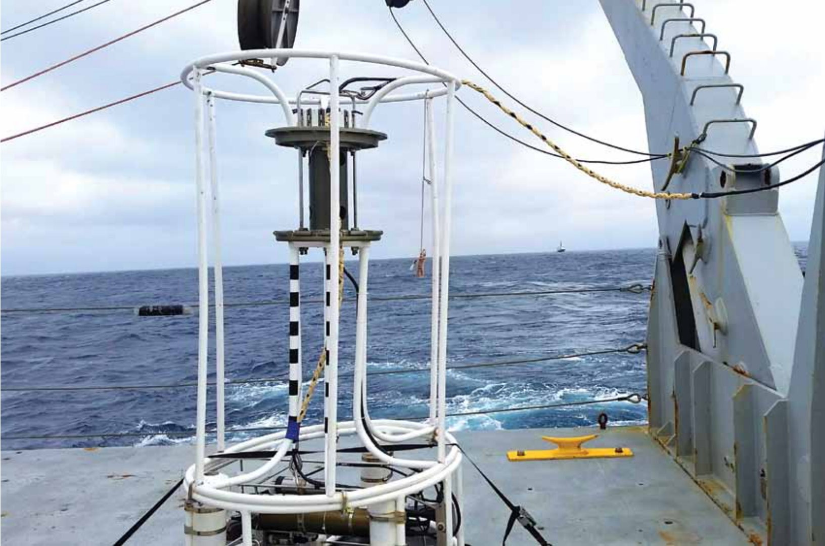
A trace metal clean instrument, on the stern of the R/V Revelle , measures salinity, temperature and depth. Photo by Heather McNair.
