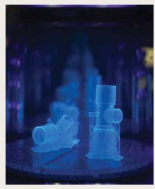
3D-printed 'exhalation ports' used in the patient circuit of a ventilator system.
