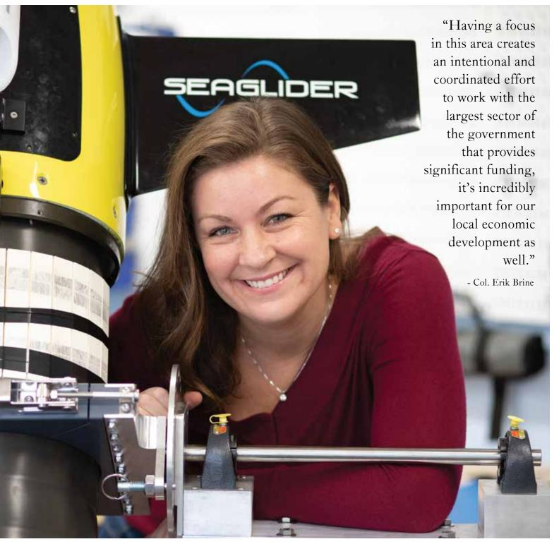
Ocean Engineering Assistant Professor Lora Van Uffelen, with the Seaglider, an autonomous underwater vehicle used for taking oceanographic measurements 1000 meters deep. Coming to the surface every few hours for satellite communication it can be in the ocean for months.
