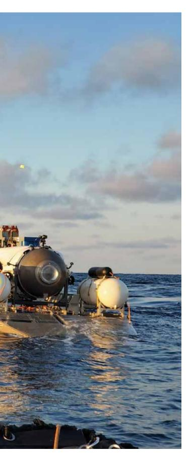
OceanGate's Titan, a five-person submersible that can dive to depths of 4,000 meters, is towed behind a research ship. (Photo courtesy of David Concannon)
