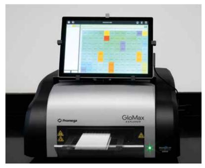
A spectrophotometer/luminometer determines how much virus present in a sample.
