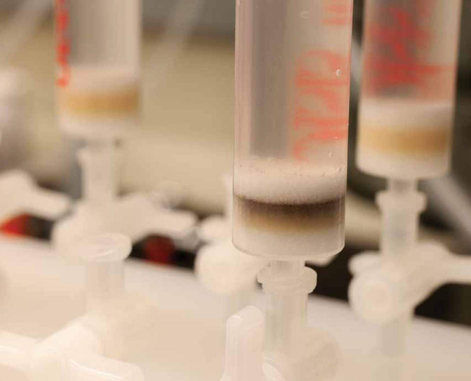
Extraction and sample cleaning-up step in preparation for trace contaminant analysis.
