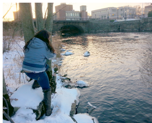
At the Blackstone River, students took water samples using polyethylene passive sampler. The sampler was retrieved 2 weeks later and sent to URI Lohmann Lab. The information was used to compare urban concentrations of POP's and PFC's along the Blackstone and other watershed areas throughout the state.
