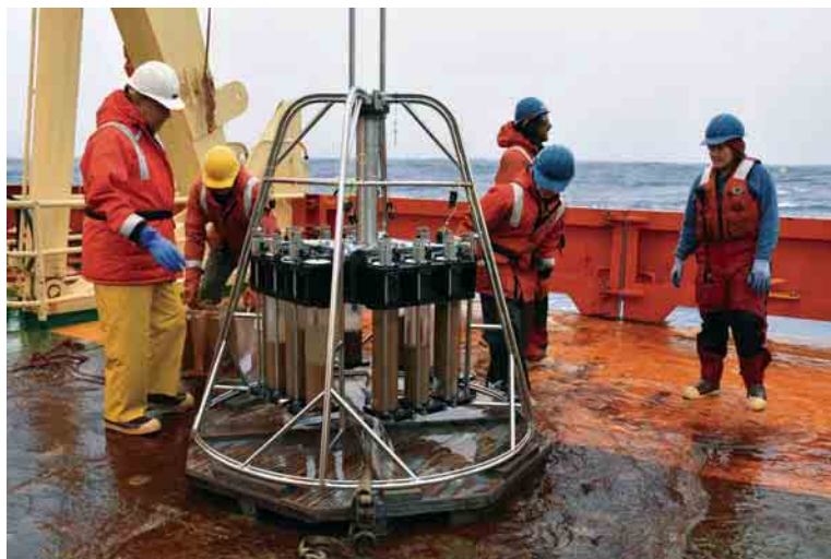
The megacorer returns to the deck and the science team begins evaluating sediment recovery at 65°S.
