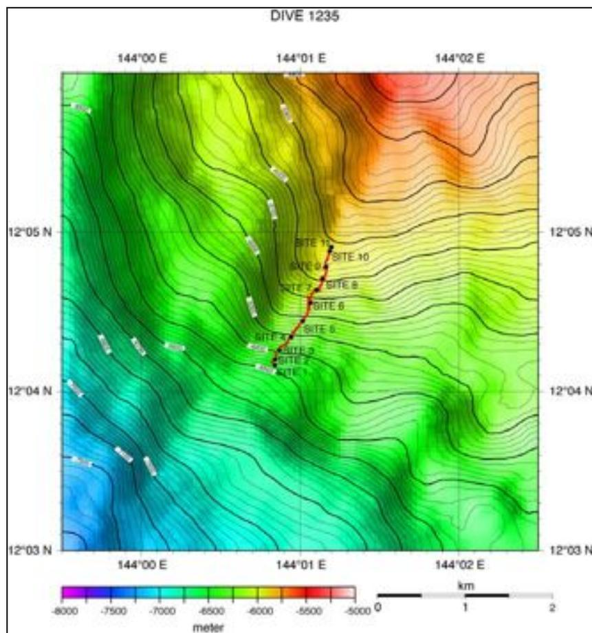
**Fig. 2.** Bathymetric map of area investigated and traverse covered by dive 6K-1235.
