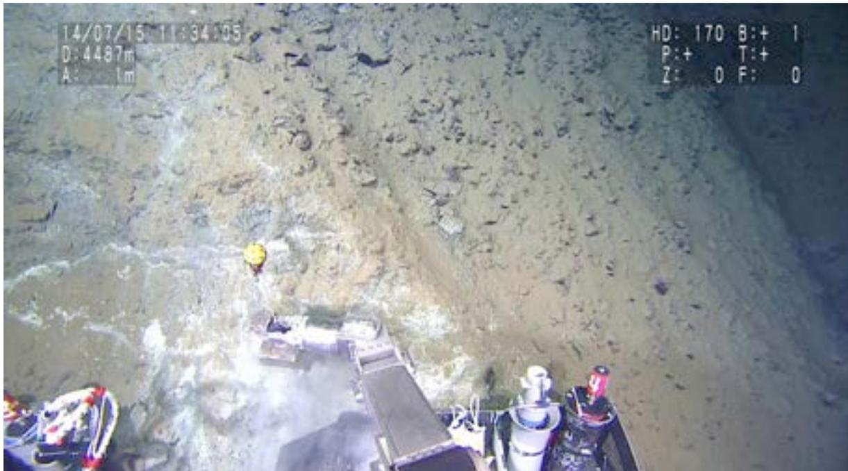
**Photo 4.** Sampling the white precipitate layer with scoop (Scoop 1) at Stop 3.
