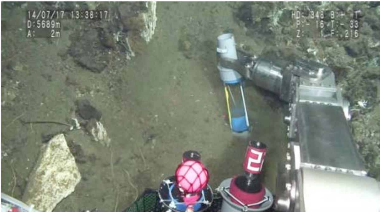
**Photo 19.** Sampling sediment with an Imai core.
