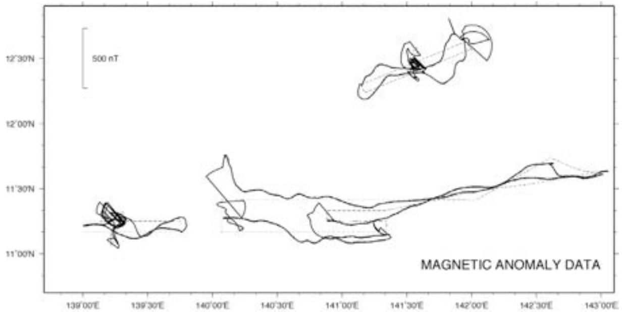
**Fig. 5. Proton magnetometer data (IGRF removed) obtained during YK14-13 cruise. Anomaly is projected perpendicular to the cruise track (dashed line).**
