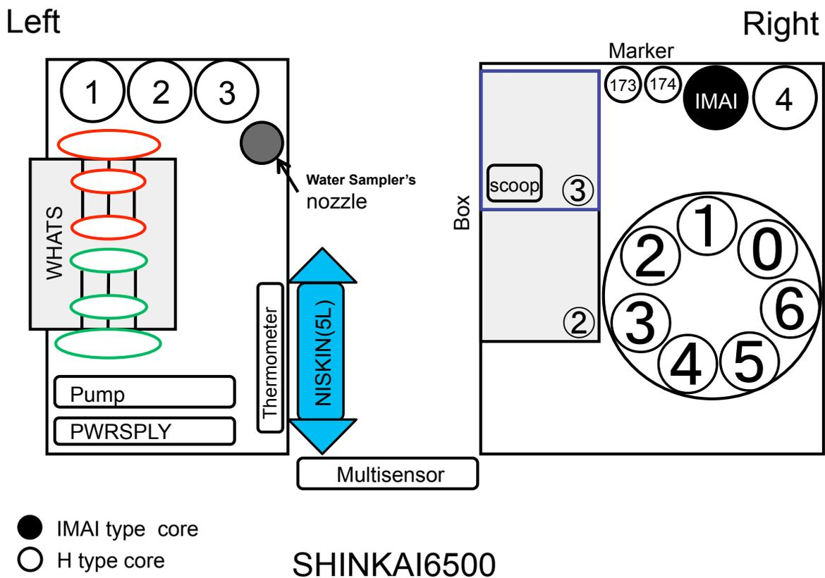
Fig. 3. Schematic illustration showing a typical payload layout employed in YK14-13 cruise.
