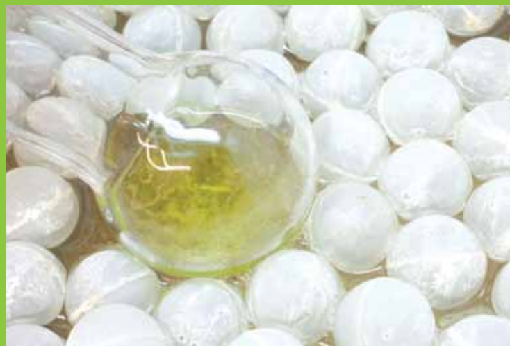
A liposome sample is being created using a rotary evaporator. The glass flask is partially submerged in a water bath and the plastic beads reduce evaporation from the bath. Liposomes are used as templates for synthesizing nanomaterials.
